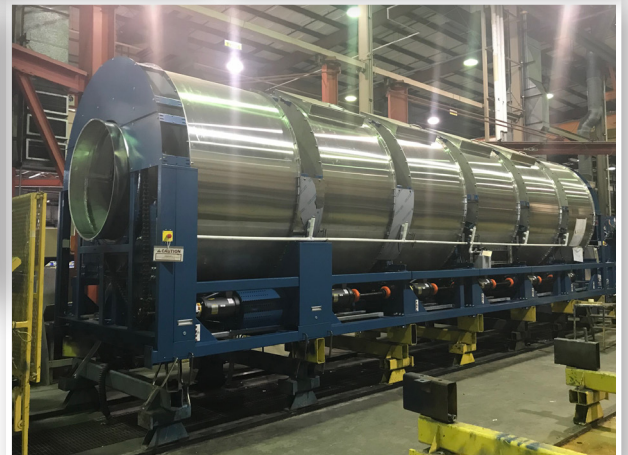
Top left to right: Concrete placement; concrete placement; outside facility. Bottom left to right: Fiberight CEO speaks to attendees at June's VIP tour; washing tunnel (separates soluble organics from the biomass pulp and fines stream, as well as to screen and separate small plastic and other contaminants not screened by the drum pulper).
